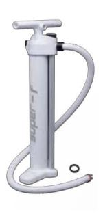
Super-F hand pump: more efficient (less effort) thanks to external aluminium tube. Pressure gauge on the lid for easy reading. Inflation port on the body to prevent kinking of the tube. In addition, the Super-F has a foldable base and the handles can be disassembled to save space in the package.
